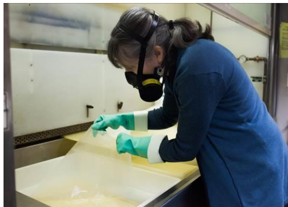
Senior Conservator Jessica Henze removing cellulose acetate lamination in a solvent bath.
