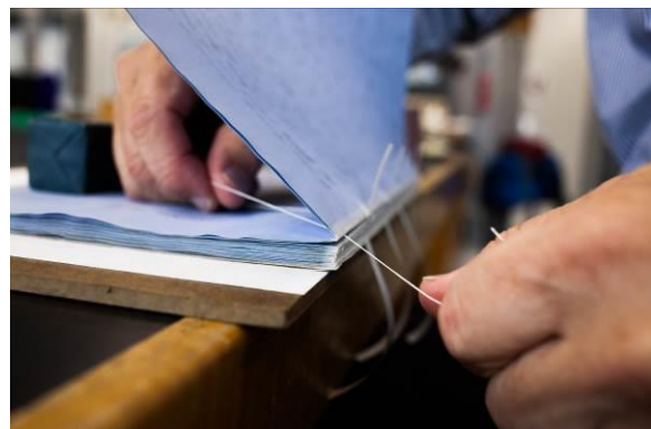
The text block is resewn using linen thread. Hand sewing is stronger and less damaging than machine sewing.
